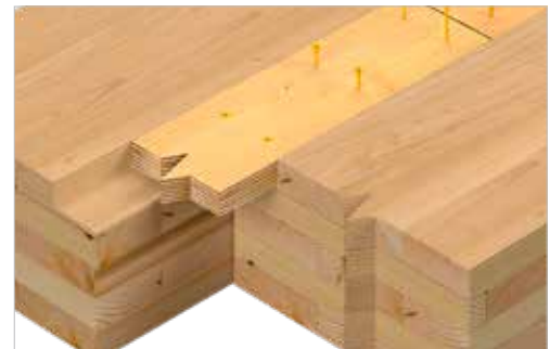
SWC screw installed in a CLT spline.
